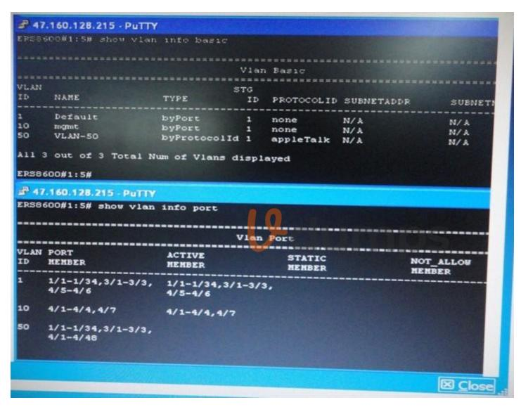
After checking the VLAN configuration using the show vlan info basic and the show vlan info port commands, there are no ACTIVE MEMBER ports for VLM4-50. What is causing this problem?
