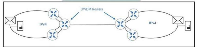
Refer to the exhibit. An engineer is planning an IPv4 to IPv6 migration solution for a customer. The routers in the network can support IPv4 and IPv6, except for the DWDM routers. The DWDM routers provide a Layer 2 link in which the routers peer directly with each other across a DWDM circuit. The circuit also provides connectivity between the mail servers. Which IPv6 migration technique must the engineer deploy?
