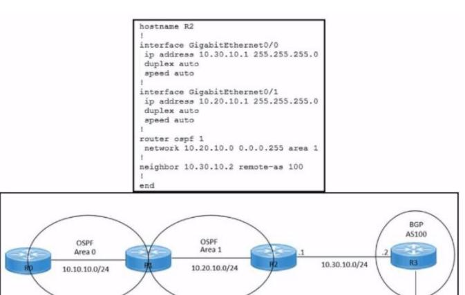
Refer to the exhibits. An engineer must redistribute IBGP routes into OSPF to connect an on-premises network to a cloud provider. Which command must be configured on router R2?
