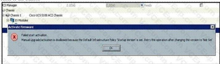
Cisco UCS Manager is being upgraded using the Auto Install feature, but the FSM fails. Which action resolves the issue?
