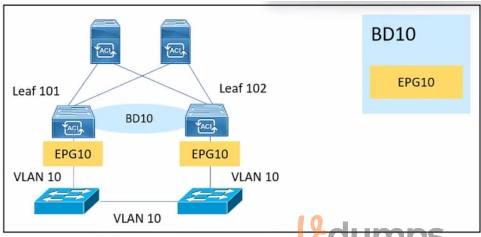
An engineer is implementing a BPDU filter on external switch interfaces That face the Cisco ACI fabric to prevent excessive TCNs from impacting the fabric. Which Configuration must be applied on Cisco ACI to avoid a Layer 2 loop?
