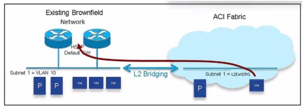
An engineer must migrate workloads from the brownfield network to the Cisco ACI fabric. The VLAN 10 default gateway remains in the router located in the brownfield Network. The bridge domain has already been associated with L2Out. Which two actions must be taken to migrate the workloads? (Choose two.)
