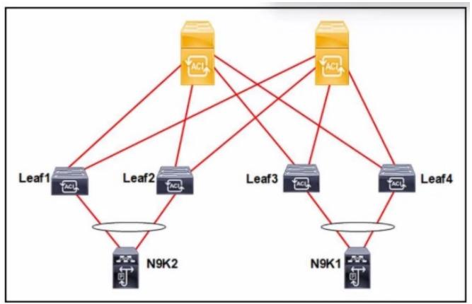
The Cisco ACI fabric is built with L2Out to the N9K1 and N9K2 switches. The switches run the RSTP protocol. The requirement is for the Cisco ACI fabric to detect 5 from the N9K and for the fabric to be protected against loops. Which set of actions must be taken to meet the requirements?
