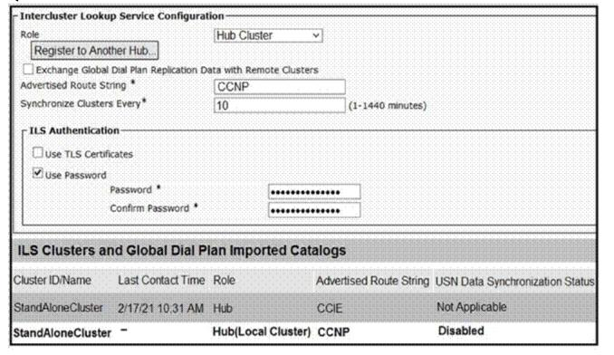
Refer to the exhibit. ILS has been configured between two hubs this configuration. The hubs appear to register successfully, but ILS is not functioning as expected. Which configuration step is missing?
