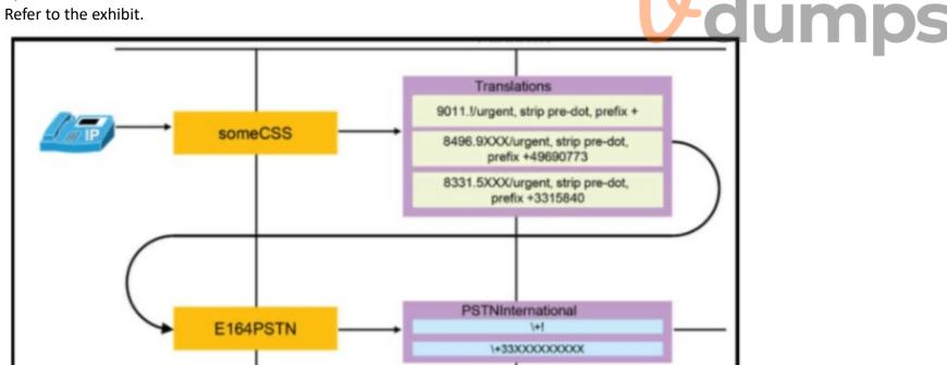
A user dials 84969010 and observes that the call is not routed immediately. The administrator notices that after matching the fixed-length translation pattern, the call hits the \+! pattern and waits for interdigit timeout What should be configured to ensure that the call routes out immediately?
