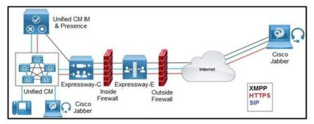
Refer to the exhibit. Which two outbound connections should an administrator configure on the internal firewall? (Choose two.)
