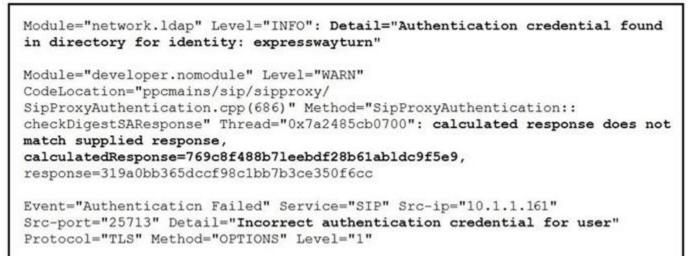
Refer to the exhibit. Mobile Cisco Jabber cannot register with on-premises Cisco Unified Communications Manager using Mobile and Remote Access. Some logs were captured on Expressway Edge. Which action corrects this problem?
