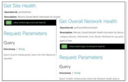
Refer to the exhibit. A developer is creating a health check monitoring script that queries information from the Cisco DNA Center platform. The script must trigger an alert if a site health statistic named accessGoodCount drops below 80 and if a network statistic named latestHealthScore is 95 or less. Drag and drop the code snippets from the bottom onto the blanks in the code to monitor the site and network health on a Cisco DNA Center platform instance. Options may be used more than once. Not
