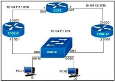
On which interfaces should VRRP commands be applied to provide first hop redundancy to PC-01 and PC-02?
