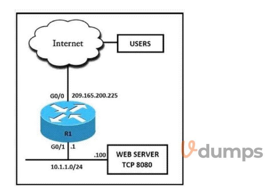
Refer to the exhibit. External users require HTTP connectivity to an internal company web server that is listening on TCP port 8080. Which command set accomplishes this requirement?
