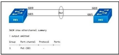
After an engineer configures an EtherChannel between switch SW1 and switch SW2, this error message is logged on switch SW2.
