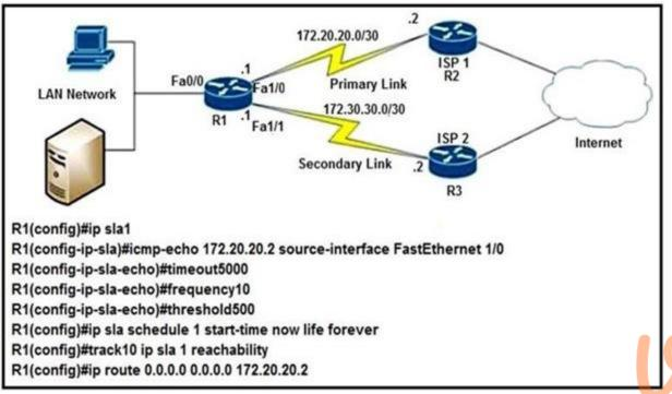
After implementing the configuration 172.20.20.2 stops replaying to ICMP echoes, but the default route fails to be removed. What is the reason for this behavior?
