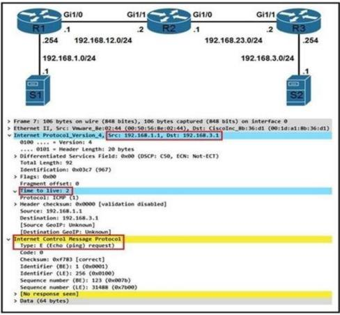
Which troubleshooting a routing issue, an engineer issues a ping from S1 to S2. When two actions from the initial value of the TTL? (Choose two.)
