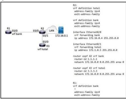
Refer to the exhibit. Which configuration must be applied to R1 to enable R1 to reach the server at 172.16.0.1?
