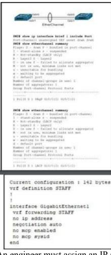
An engineer must assign an IP address of 192.168.1.1/24 to the GigabitEtherenet interface. Which two commands must be added to the existing configuration to accomplish this task? (Choose two.)
