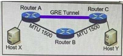
MTU has been configured on the underlying physical topology, and no MTU command has been configured on the tunnel interfaces. What happens when a 1500-byte IPv4 packet traverses the GRE tunnel from host X to host Y, assuming the DF bit is cleared?
