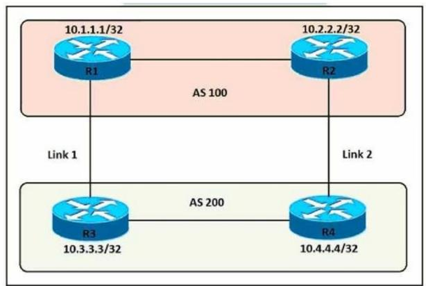
An engineer must ensure that all traffic leaving AS 200 will choose Link 2 as an entry point. Assuming that all BGP neighbor relationships have been formed and that the attributes have not been changed on any of the routers, which configuration accomplish task?
