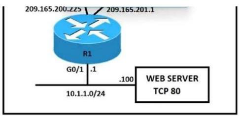
An engineer must configure static NAT on R1 lo allow users HTTP access to the web server on TCPport 80. The web server must be reachable through ISP 1 and ISP 2. Which command set should beapplied to R1 to fulfill these requirements?
