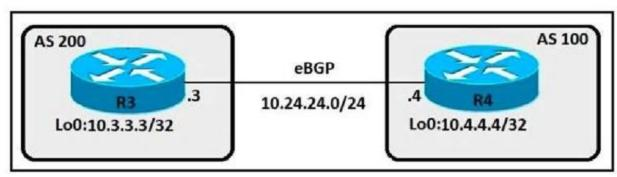
An engineer must establish eBGP peering between router R3 and router R4. Both routers should use their loopback interfaces as the BGP router ID. Which configuration set accomplishes this task?
