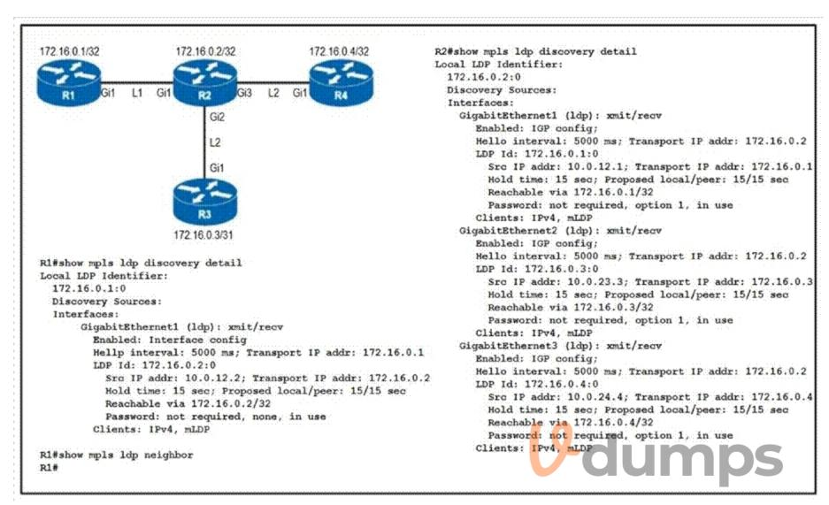
An engineer began to configure LDP between R1 and R2, but R1 and R2 cannot yet establish an LDP TCP connection. Which additional task must be completed to finish the implementation?
