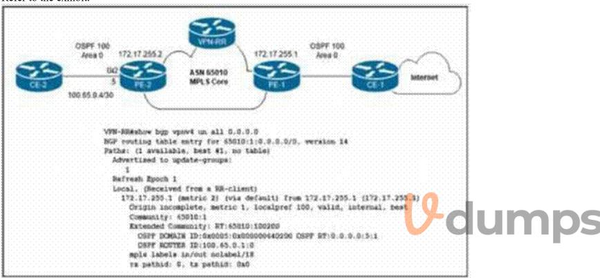
The network engineer who manages ASN 65010 is provisioning a customer VRF named CUSTOMERABC on PE-2. The PE-CE routing protocol is OSPF Internet reachability is available via the OSPF 0 0 0.0/0 route advertised by CE-1 to PE-1 In the customer VRF Which configuration must the network engineer Implement on PE-2 so that CE-2 has connectivity to the Internet?
