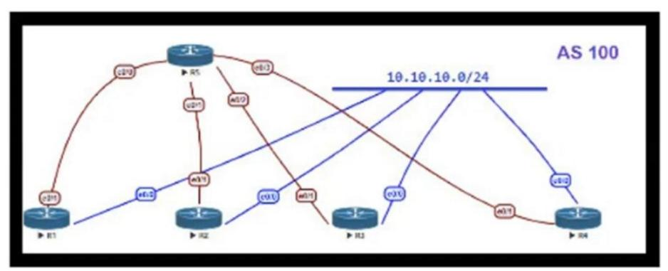
OSPF is running as the IGP to provide reachability to all AS100 networks R3 and R4 are the current ABRs at the boundary of OSPF Area0 and Areal Now BGP must be deployed within AS 100 because it will be receiving Internet routes from its eBGP peers (the service provider) connected to R1 and R2 What is an optimal solution for this deployment to configure BGP relationships and redistribute BGP learned routes into OSPF?
