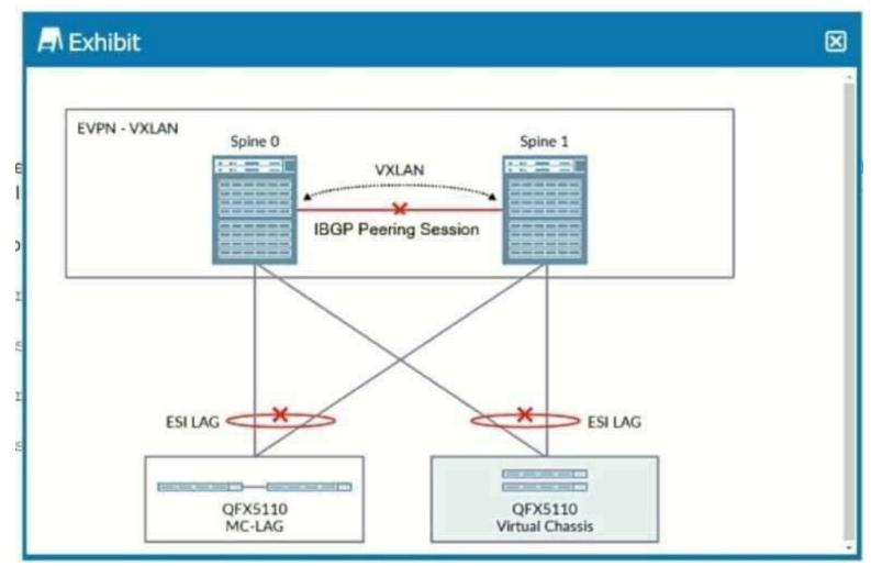
you have a data center in which only the spine devices are using EVPN and VXLAN. The leaf nodes are multihomed in active-active mode to the spine nodes through ESI LAG interfaces. In this design, a link failure on the interface connecting the spine nodes would also cause all traffic from the spine to the leaf nodes to drop.
