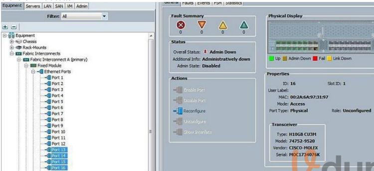
A client has added a new chassis and connected ports 13 through 16 on both fabrics to the I/O modules. The client has verified the Twinax cabling. The Chassis/FEX Discovery Policy is set to 4 Link. However, the new chassis still fails the discovery process.
