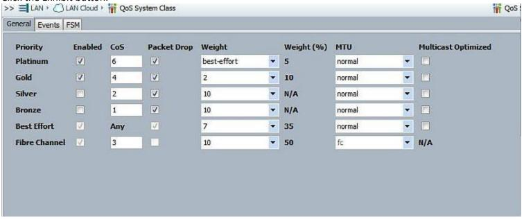
Your client explains that they are not able to communicate with virtual machines in the UCS using a packet size of 9000. Referring to the exhibit, what needs to be corrected to resolve the network problem?
