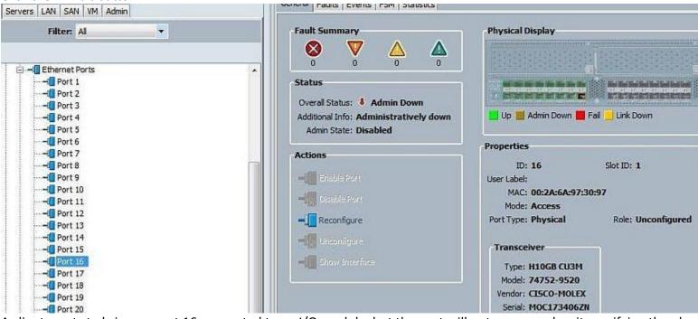
A client wants to bring up port 16 connected to an I/O module, but the port will not come up despite verifying the physical cabling of the Twinax cables.
