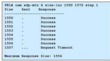
E-pipe 100 is using an SDP with an LSP that uses the path shown (PE1-PE2-PE3-PE4). Based on the OAM command output, which of the following is FALSE?
