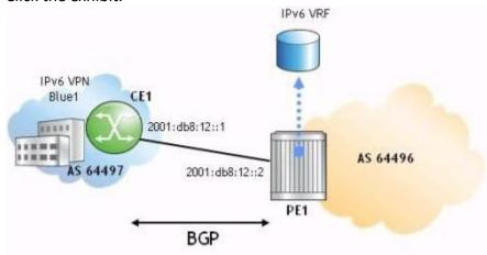
Part of a 6VPE deployment is shown in this exhibit. Which of the following is the correct configuration and context on PE1 for a BGP peering session with CE1?
