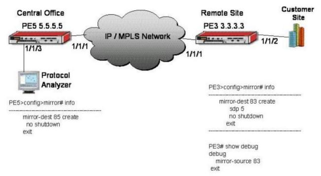
Assuming the customer only needs to monitor traffic from PE3 to the customer site, what three items are missing from PE3's configuration? (Assume that the IP/MPLS network structure between the local and remote PEsis in place.)
