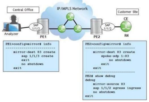
PE1 and PE2 are Nokia 7750 SRs. What needs to be added to PE1's configuration to mirror traffic between PE2 and the customer site?
