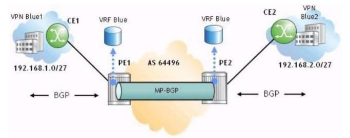
Assuming CE1 exports its system address using BGP, is a routing policy required on PE1 to advertise CE1's system address to PE2?
